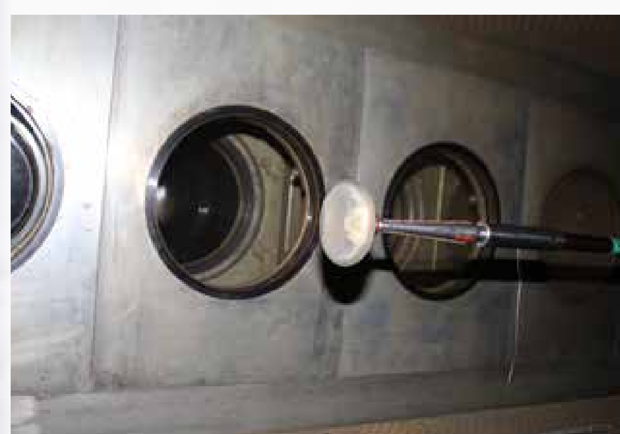
Figure 3: Mini-1 mock-up inside wind test chamber. Picture: Lavochkin.
