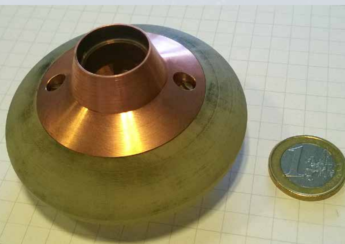
Figure 3: Wind tunnel test mock-up. Picture: FMI.
