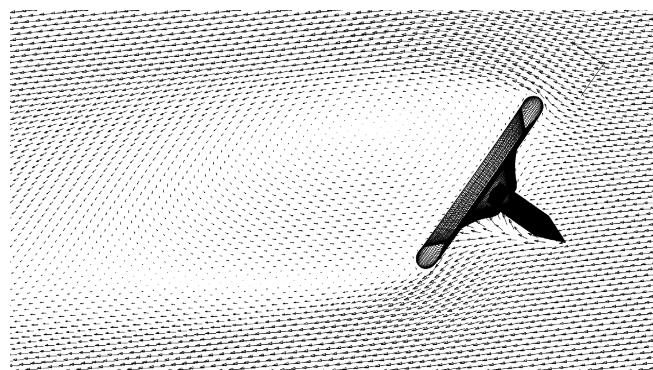
Velocity vectors around the MetNet AIBU configuration. Angle of attack = 35 degrees; Ma=0.7, Re=180000. Time averaged calculation. Picture/simulation: M.Palin (Aalto) / Finflo Ltd.
