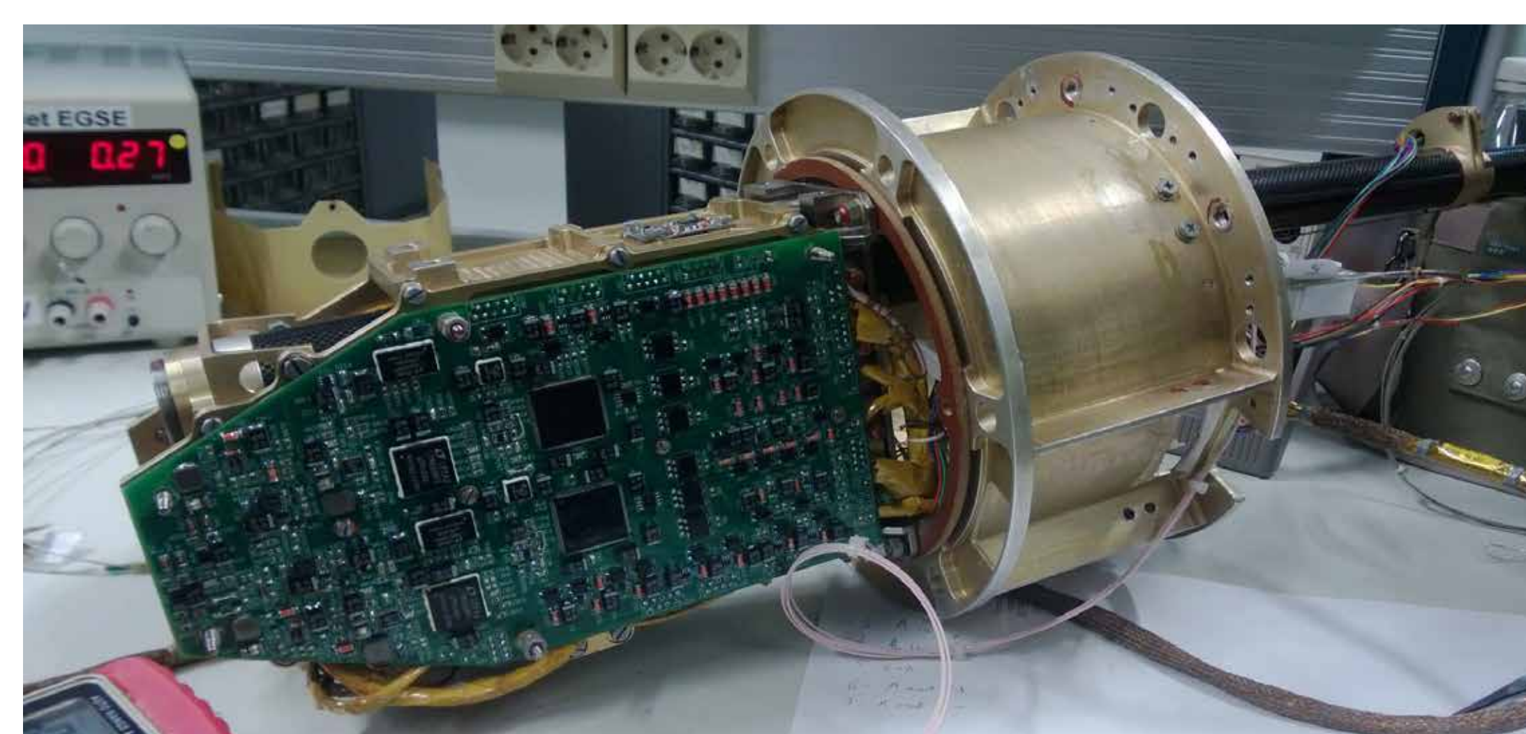
MetNet Lander payload bay and computer in tests in FMI. Picture: FMI.
