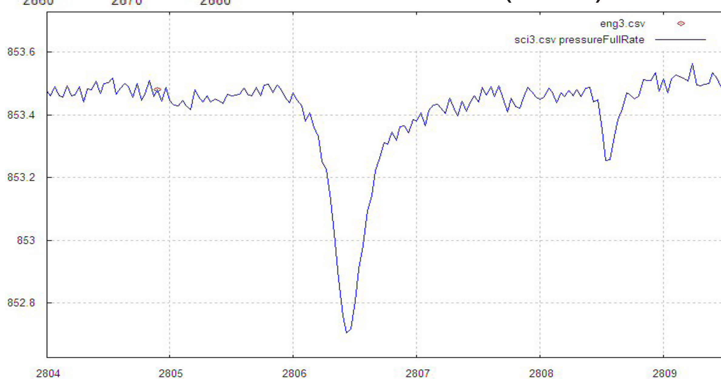
Pressure drops caused by dust devils detected by the FMI Phoenix Pressure device in Autumn 2008.
