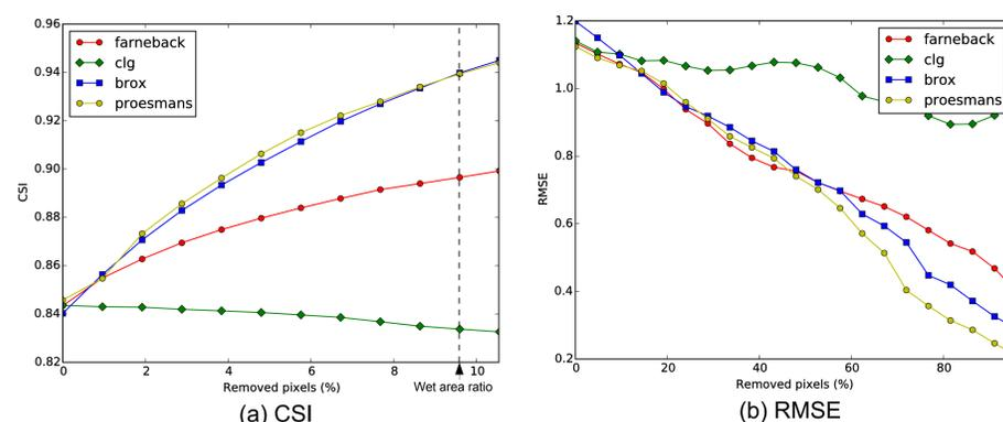
Figure 3. CSI and RMSE curves for advection-based temporal interpolation, Case 5.
