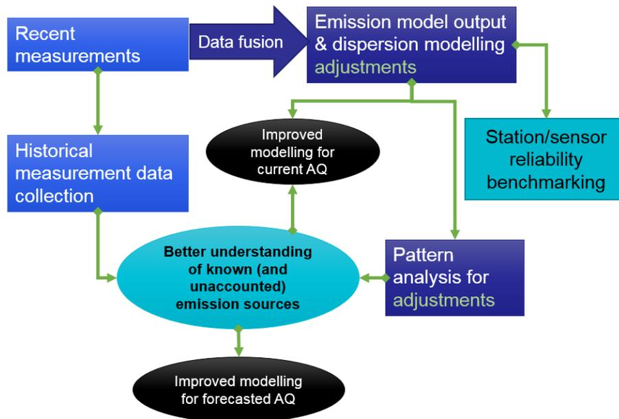
**Figure 2: The learning process of Enfuser data fusion. Based on the model predictions at measurement locations, data fusion is used to adjust dispersion modelling parameters and local emission source outputs. Over a longer time period, statistical analysis of the hourly adjustments can be used to reveal patterns that facilitate model improvements, especially for the used local emission inventories. As a by-product, measurement device reliability benchmarking over time is available.**
