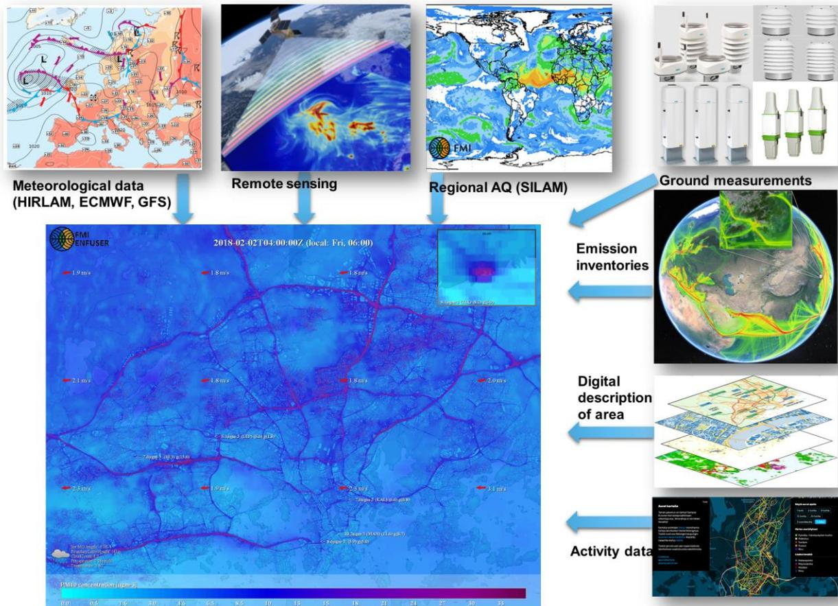
**Figure 1: The core components of FMI-ENFUSER modelling system, which utilizes latest sensor observations, meteorological data and regional air quality forecast in the production of high resolution AQ heatmaps for the current and future situation in urban locations. GIS-datasets and emission inventories together with archived concentration time series are used for the calibration of the model.**
