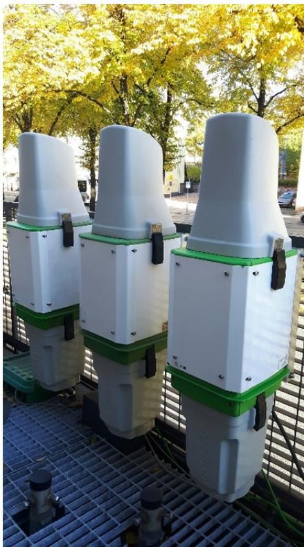
**Figure 4.3.1.** Co-located precision measurement configuration. The AQ Urban (Mäkelänkatu unit) located in the middle was used as a reference. Photo © HSY / Anssi Julkunen.
