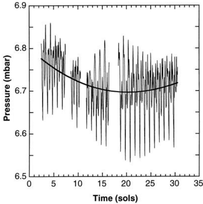
Fig.3A. Time-averaged pressure for the first 30 sols. Averaging basically 3-minute sessions 51 sessions per day. The resulting points were connected by straight lines, except for from 12 to 15 Sol, where the lack of data for 8 hours enterprisesales splines. Large gaps in 1,8,11, and 17 Saul caused reboots and connection issues. The long-term trend (solid curve) is represented by fitting a polynomial of 3rd order.
