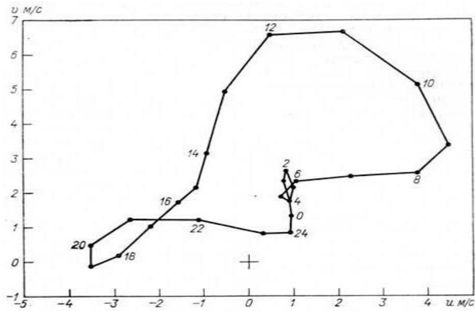
Fig. 7. The hodograph of the vector of the horizontal wind speed according SA "Viking-1" in 20 Martian days. The numbers at the locus designated hours of the day counted from midnight,  $u$ ,  $v$  — West and South wind components, respectively.
