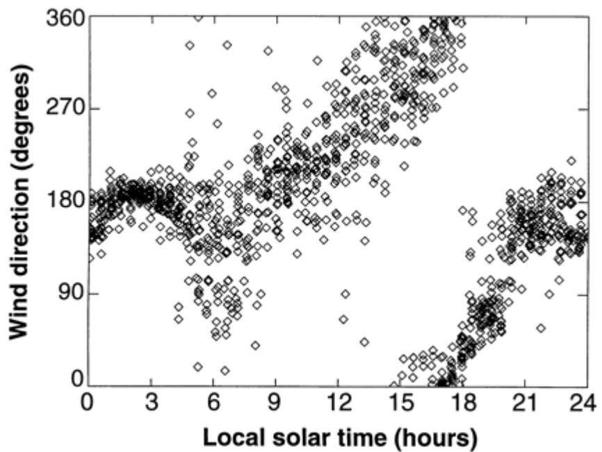
Fig.6. Time-averaged wind direction for the first 30 sols as a function of local solar time. Each point represents the average for 3 minutes. Marking directions: 0° and 360° (North), 90° (East), 180° (South) and 270° (West).
