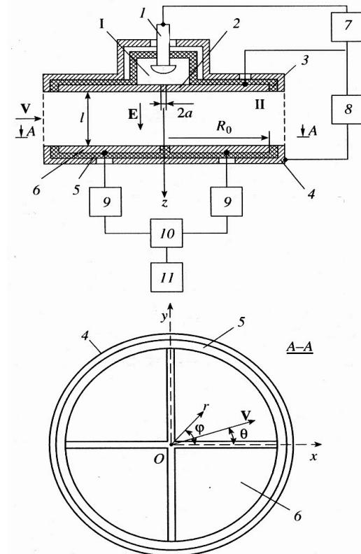
Gas discharge anemometer.
