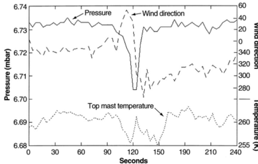
**Fig.8. Changes of pressure, temperature and wind speed associated with a small vortex that passed over the landing site Pathfinder. The measurements were performed with an interval of 4 seconds.**
