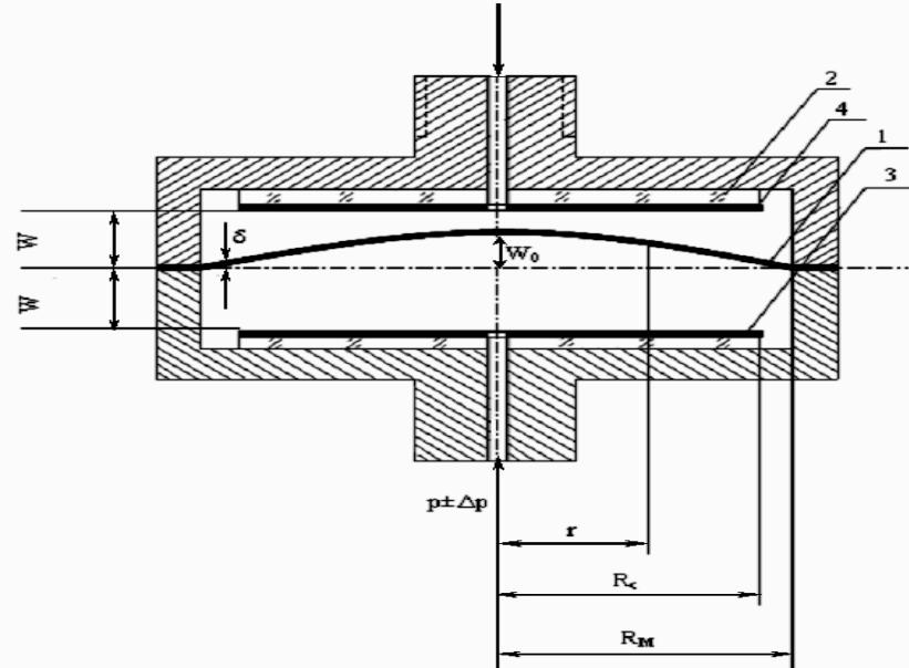
The sensing element of the pressure sensor:
