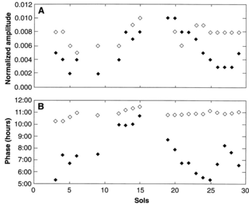
**Fig.7.** (A) the amplitude of the diurnal (black diamonds) and semi-diurnal (light rhombs) of the pressure waves for the first 30 sols. The amplitude is normalized relative to the average pressure for the day. (B) Phase in LST, the diurnal (black diamonds) and semi-diurnal pressure waves.
