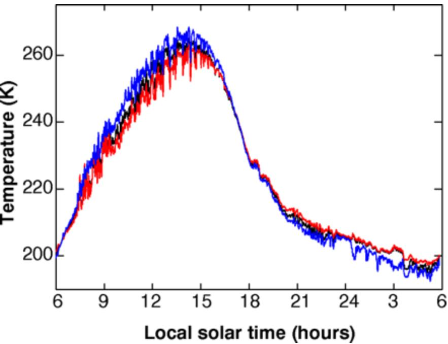
**Fig.4.** Daily variations of atmospheric temperature, measured by thermocouples at the top (red), middle (black) and bottom (blue) mast 06.00 LST of the 25th Sola 0600 LST 26th Sola. Thermocouples located at 100, 50 and 25 cm above the plane of the solar panels. The measurements were performed every 4 s, but the chart data is averaged over the interval of 2 minutes to reduce fluctuations.
