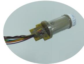
Humicap® humidity sensor chip is a capacitive sensor. It contains an active polymer film that changes capacitance as function of relative humidity and temperature. **The capacitance is also affected by CO<sub>2</sub> gas, and the magnitude of the effect is dependent on both temperature and pressure.**
