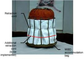
Figure 3-5 MML prototype (folded)
